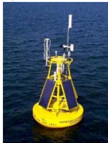
The new buoy system undergoing tests off the WHOI dock. The foam flotation collar is the basic buoy hull. On top of the tower the satellite receiving antenna (on right) and transmitting antenna (on left) are mounted as far apart as possible.
