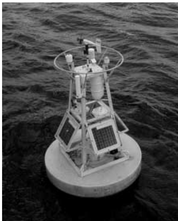
Figure 1. The GLOBEC buoy with meteorology sensors visible on the top of the tower. The R.M. Young Anemometer is highest; behind it is the Gill radiation shield holding the Rotronics air temperature and relative humidity sensor. On the left is the Eppley long-wave radiation; on the right is the Eppley short-wave radiation sensor. The small dark sensor on the front of the top plate of the tower is the LiCor cosine PAR sensor.
